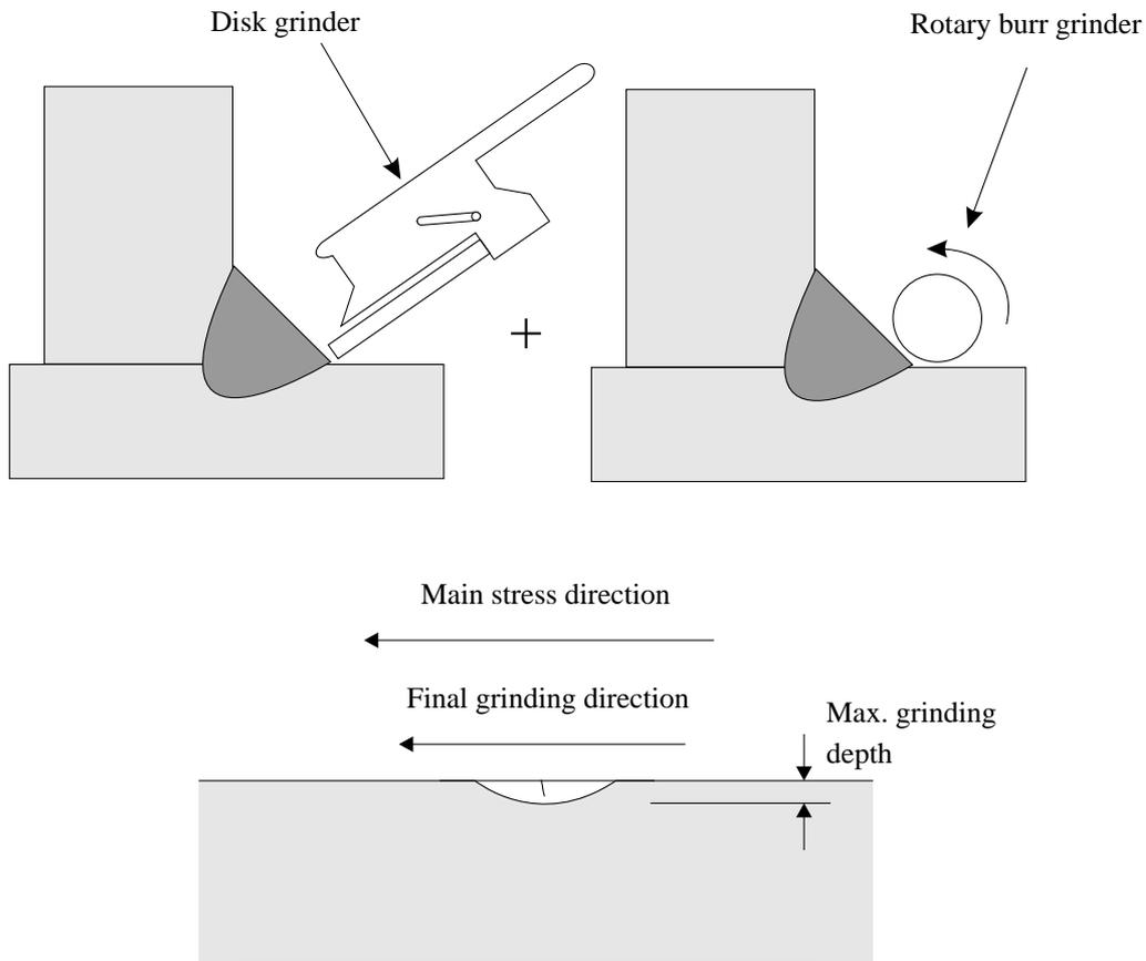
Fig 6.9 Grinding
