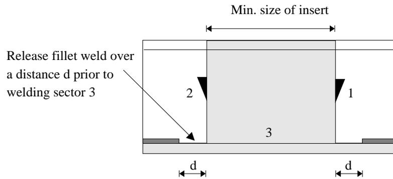
Fig 6.4 Welding sequence for inserts of stiffeners
