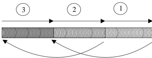
Fig 6.8.c Welding sequence for cracks with length less than 300 mm
