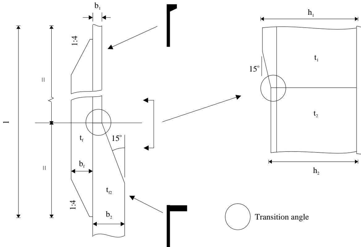
Fig. 6.5 Transition between inverted angle and bulb profile
