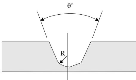
Fig. 6.8.d Groove preparation
